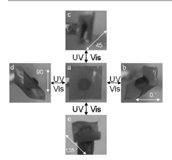
Figure 2. Photographic images of precise control of bending direction by polarized light; From (b) to (e), photomechanical bending of PNLCP films. Arrows in the figures indicate the direction of polarized light; (a) Photomechanical unbending induced by visible light (>520 nm).
