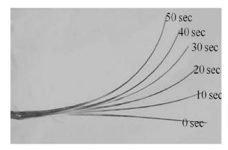
Figure 1. Superimposed microphotographs of PNLCP fiber under UV irradiation.
